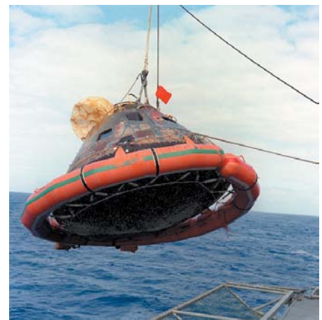
Figure 4.1.7-21. Ablative Cooling. The bottom side of the Apollo re-entry capsule shown here was coated with a ceramic material that literally melted away during re-entry. As it melted, it took away the fierce heat and kept the astronauts safe and comfortable. (Courtesy of NASA/Johnson Space Center)
