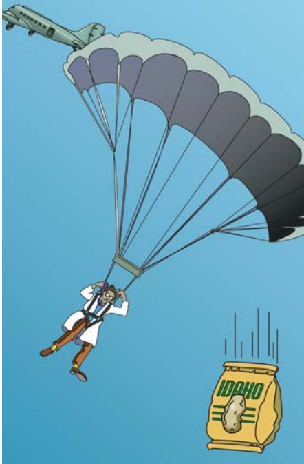
Figure 4.1.7-7. Changing BC. With his parachute open, the skydiver greatly increases his area, A , and drag coefficient, C_D , thus decreasing his ballistic coefficient, BC , and slowing down much faster than the potatoes.
